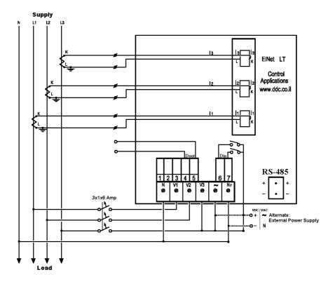
Figure 2.3 Schematic Wiring Diagram "Star" connection
