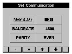
Figure 6.2 Serial Communication Setup
