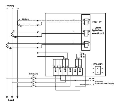
Figure 2.4 Schematic Wiring Diagram "Delta" connection
