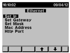
Figure 6.3 Ethernet Communication Setup
