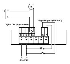
Figure 2.5 Digital In \ Digital Out wiring example
